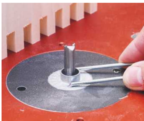
▲ By moving the guide bush in small increments the fit of the joint can be adjusted
